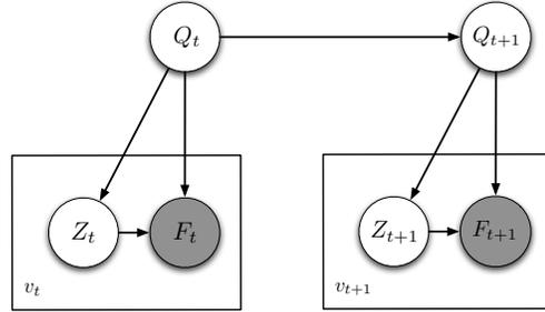
**Fig. 2.** Graphical Model of the N-HMM.  $\{Q, Z, F\}$  is a set of random variables,  $\{q, z, f\}$  their realization and  $t$  is the index of time. Shaded variable indicates observed data.  $v_t$  represents the number of draws at time  $t$ .
