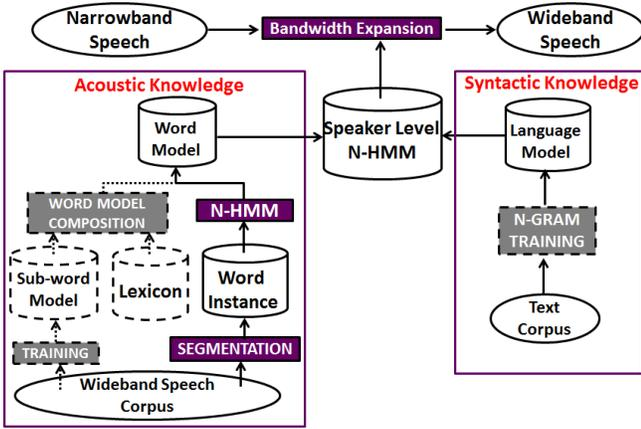
**Fig. 3.** Block diagram of the proposed system. Our current implementation includes modules with solid lines. Modules with dashed lines indicate possible extensions in order to make the system more feasible for large vocabulary BWE.
