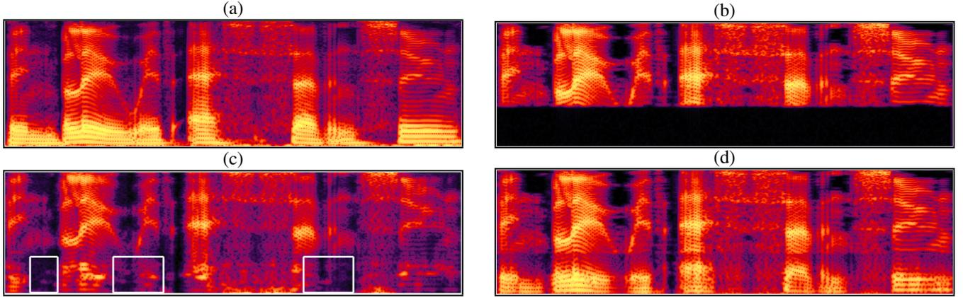
**Fig. 4.** Example of speech BWE. The x-axis is time and y-axis frequency. a) Original speech; b) Narrowband speech. c) Result using the PLCA; Regions marked with white-edge boxes are regions in which PLCA performed poorly. d) Result using the proposed method.
