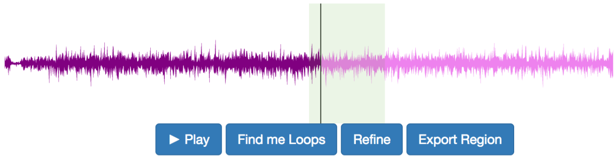
Figure 1. Interface for LoopMaker. It can automatically create loops using the Find me Loops button. It can assist users in creating loops in semi-automatic mode using the Refine button after users roughly select a region using the cursor.
